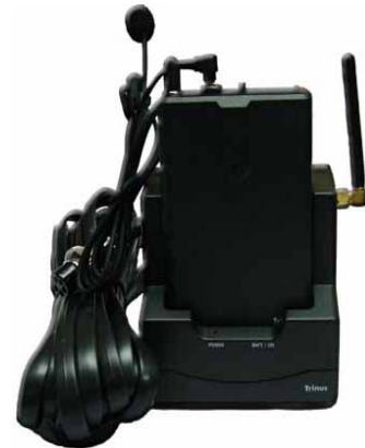
Figure 8 : 900MHz Spread Spectrum Transmitter & Reciever / Charging Base
